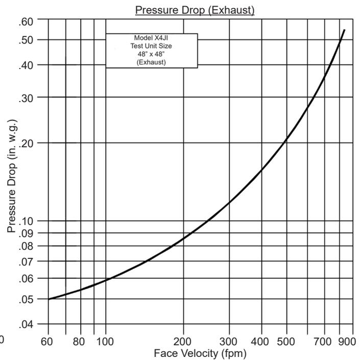
Typical performance for Model X4JI combination louver, without the use of blade linkage, counterweights, and screens.
