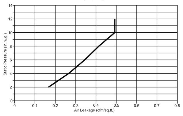
Air leakage chart is based upon independent air leakage tests conducted by Architectural Testing Laboratory. The outopening model of a 24" x 60" AHF-Z2I was tested. Tests were in accordance with ASTM E 283-91 "Determining the Rate of Air Leakage through Exterior Windows, Curtain Walls, and Door under Specified Pressure Differences Across the Specimen". Cesco Products recommends using out of opening doors for draw through applications and in opening (IO) for blow through applications.
